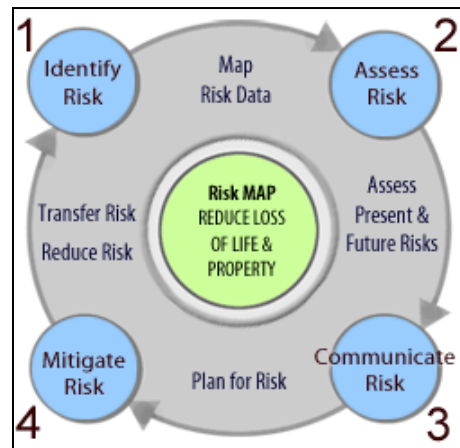
Figure 5. FEMA’s Risk MAP (Mapping, Assessment & Planning) lifecycle illustrates the process of identifying risks by utilizing flood hazard mapping and data
